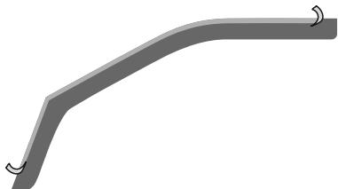
2. Remove the protective liner from the tape on the deflector.
