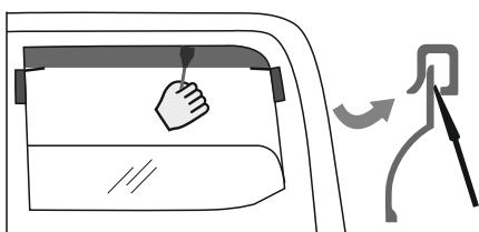
6. To ensure better installation of the deflector and better adhesion between the tape and the surface of the rubber seal, it is strongly recommended that you use the plastic blade, moving it slowly between the window's inner rubber seal and the deflector.
