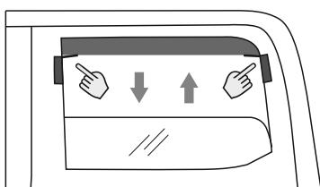
5. Place the fastening brackets onto the outside part of the rubber seal as shown in the picture. The fastening brackets must touch the lower part of the deflector.
