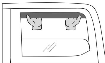
4. Immediately after installing the deflector, adjust its position by carefully pulling it outwards.
